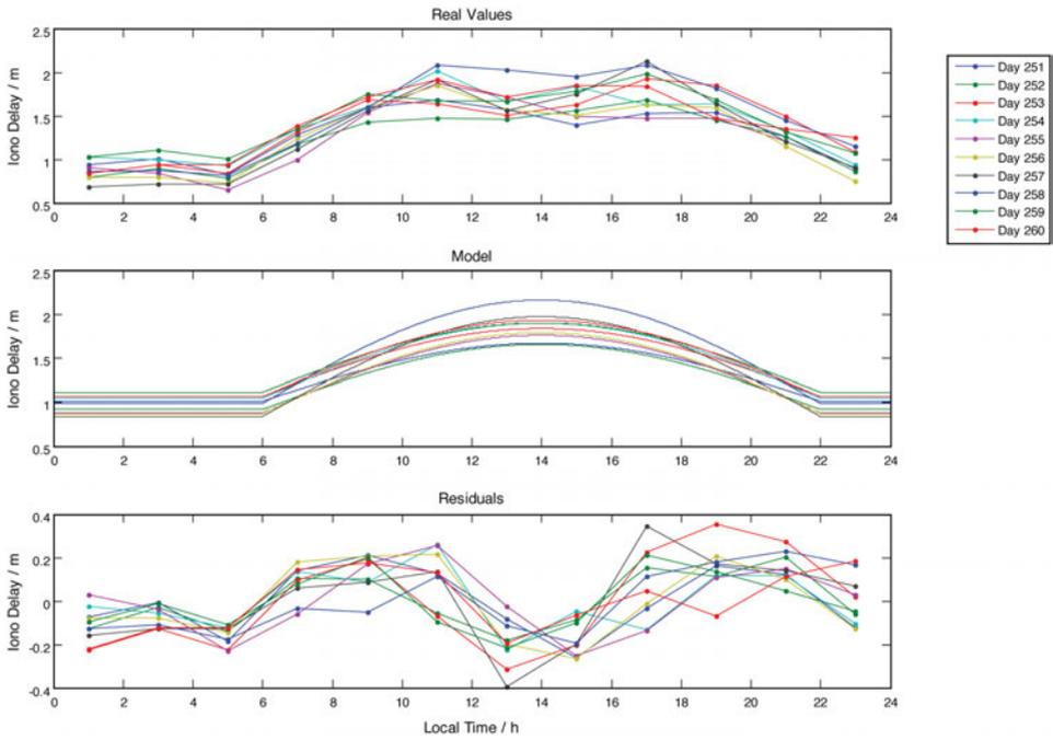
Figure 4. Composite observed GPS ionospheric delay and its components (summer-time model and residuals) in quiet space weather conditions, northern Adriatic, for days 251–260, Summer 2007 (y-axis in [m], x-axis in [h], local time).
