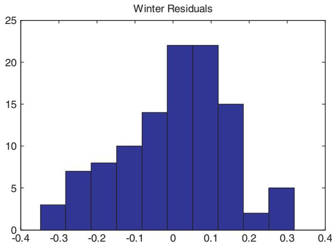
Figure 7. Histogram of residual GPS ionospheric time delay during quiet space weather conditions, northern Adriatic, days 357–365, Winter 2007 (y-axis in number of observations, x-axis in GPS ionospheric delay values in [m])
