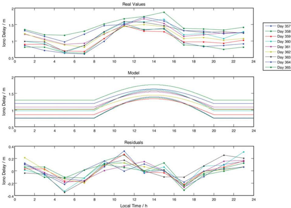
Figure 6. Composite GPS ionospheric delay and its components (winter-time model and residuals) in quiet space weather conditions, northern Adriatic, for days 357–365, Winter 2007 (y-axis in [m], x-axis in [h], local time.)
