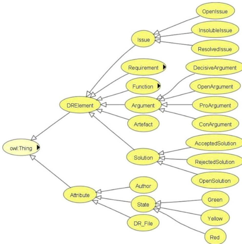
Fig. 3. Main class hierarchy of design rationale ontology.
