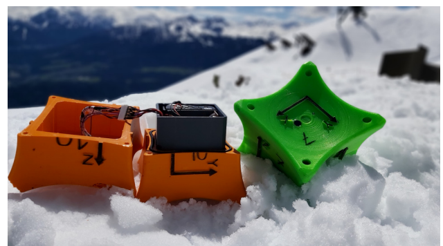
Figure 2. The figure displays two generation II AvaNodes employed in the experiments, namely AvaNode C10 (orange) and AvaNode C07 (green). AvaNode C10 has a density of \rho = 415 \text{ kgm}^{-3} , while C07 represents a density variation with a density of \rho = 688 \text{ kgm}^{-3} . It is important to note that the density is solely determined by the housing of the AvaNode, while the internal hardware remains consistent for both devices.
