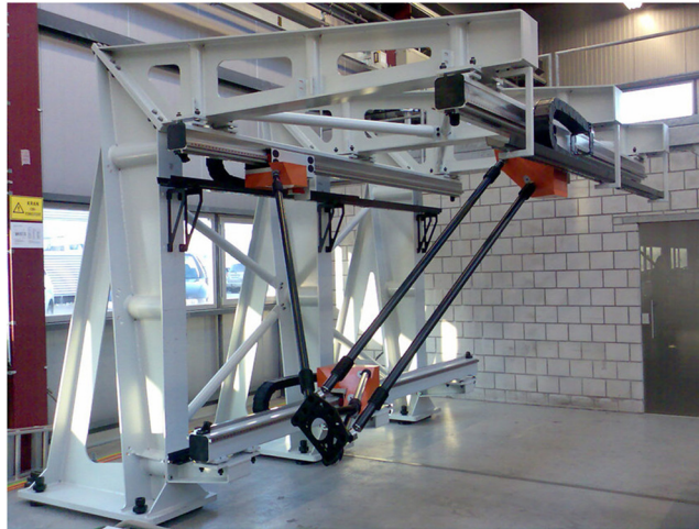
Fig. 2. 3-Degree-of-freedom (DoF) Gantry-Tau mechanism. 24
