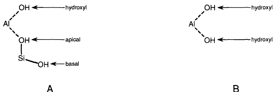
Figure 1. Schematic models of reactive groups at the edge face of kaolinite: A) Schofield and Samson (1953) and B) Muljadi et al. (1966).
