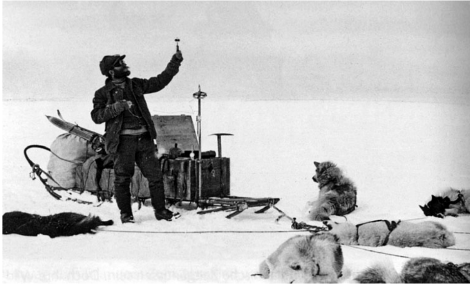
Fig. 7. De Quervain checking wind velocity with a hand-held anemometer (ETH-Zürich, Image Archive, Dia_297-0071).
