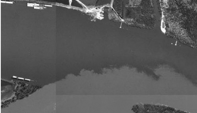
Figure 4.15 Confluence of the silty Missouri and clearer Mississippi rivers near St. Louis, MO, showing spatially growing instability. Image courtesy United States Geological Survey (USGS).
