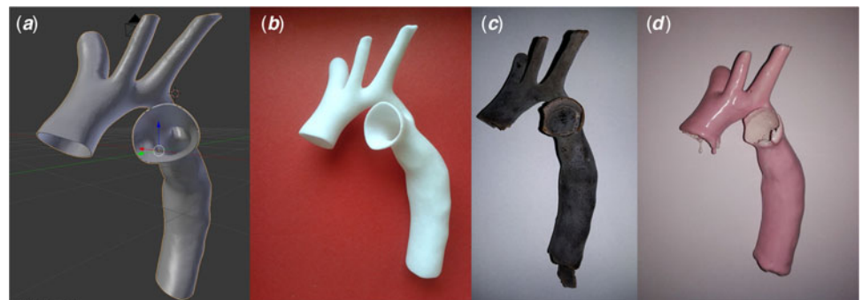
Figure 2. Consecutive stages of silicone phantom creation. (a) Virtual model – result of angio-CT data processing. (b) 3D-printed, rigid hollow model. (c) Wax core ready to apply silicone coating. (d) Hollow elastic phantom before simulation.
