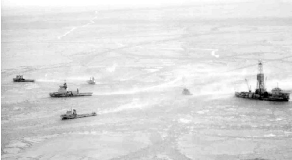
Figure 1. Beaufort Sea drilling operations from a moored drillship, in the late 70s (from Keinonen et al., 2007).
