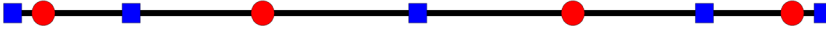
Figure 31. Solution (red circles) and flux (blue squares) points of spectral difference discretisation in the reference element ( N = 4 ).
