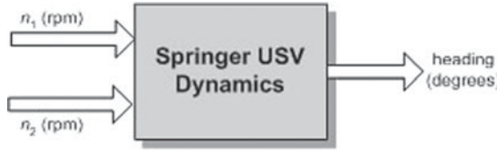
Figure 3. Block diagram representation of a two-input Unmanned Surface Vehicle (USV).
