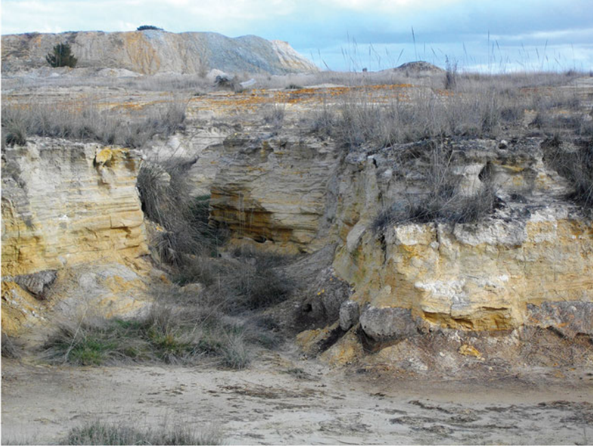
Figure 6. Mine tailings at Creswick; the tailings are the laminated deposits in the foreground; the large mound in the background is mullock, or waste material.
