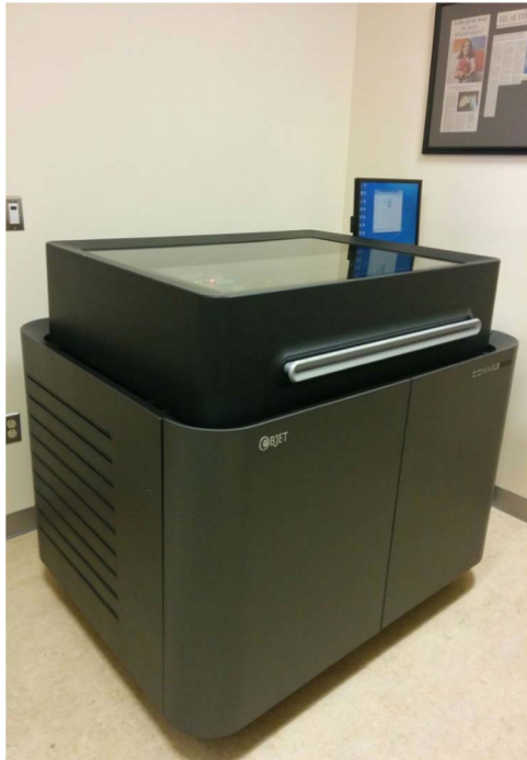
Figure 2. A three-dimensional printer at Children's National Medical Center allows creation of life-size cardiac models including complex congenital cardiac anomalies.
