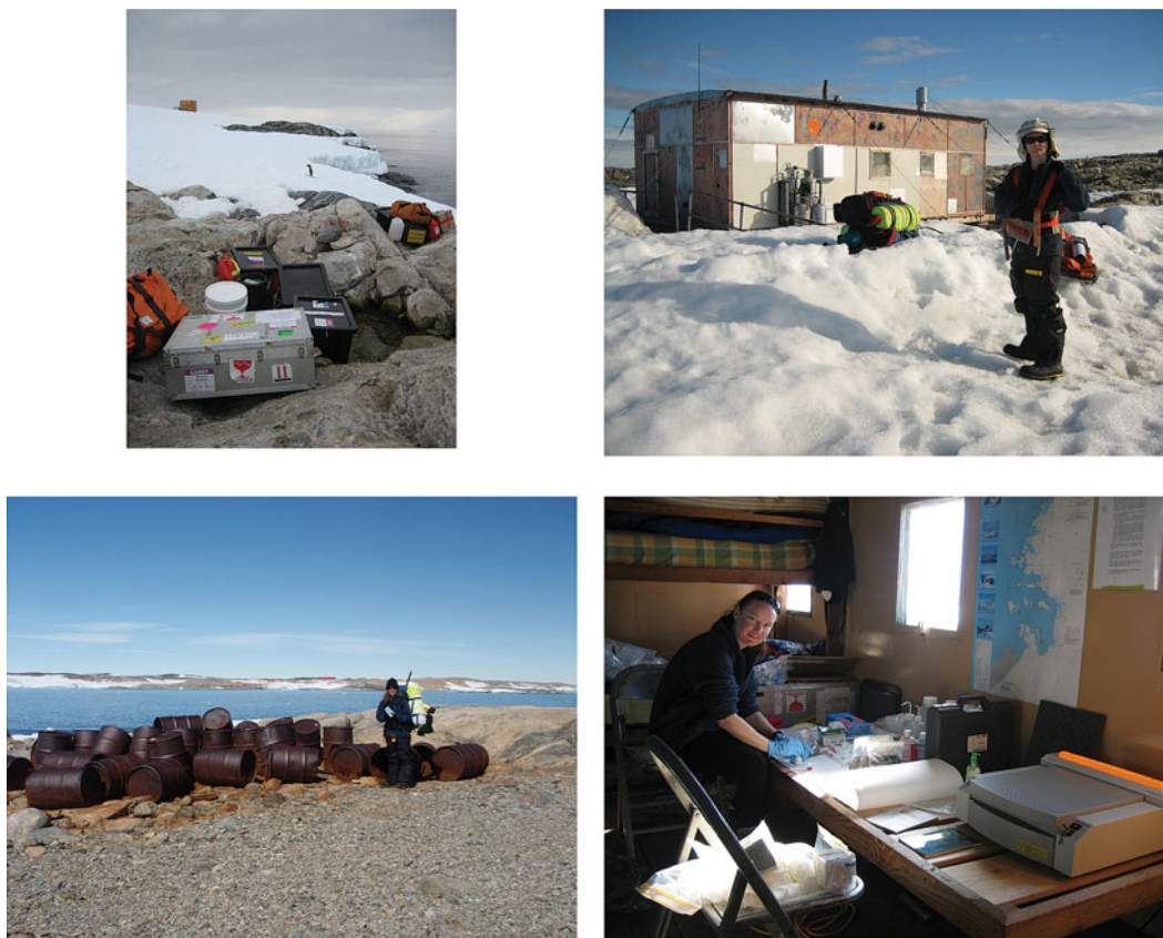
Figure 4. (Color online) Contaminated site assessment at Wilkes Station, Antarctica. Top left: Transporting the XRF to Wilkes via IRB before being carried by hand over rocks to the snow. Top right: Transporting equipment by hand-drawn sled to the field hut. Lower left: Sampling waste among rusty steel fuel drums that are over 50 years old. Lower right: On-site laboratory at a field hut. MiniPal 4 spectrometer is visible at lower right. Source of photographs: K. Fryirs.
