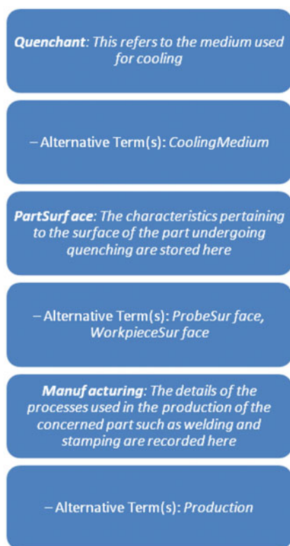
Fig. 6. A partial diagrammatic representation of the quenching ontology. [A color version of this figure can be viewed online at http://journals.cambridge.org/aie ]
