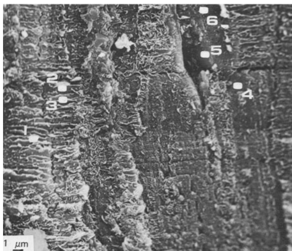
Figure 3. Magnified view of the central "A" portion of Figure 1 along a fracture surface which probably served as an avenue for impregnation by silica-bearing solutions.
