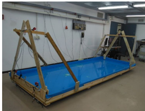
Fig. 6. Experimental setup. Water pool with Optitrack cameras.
