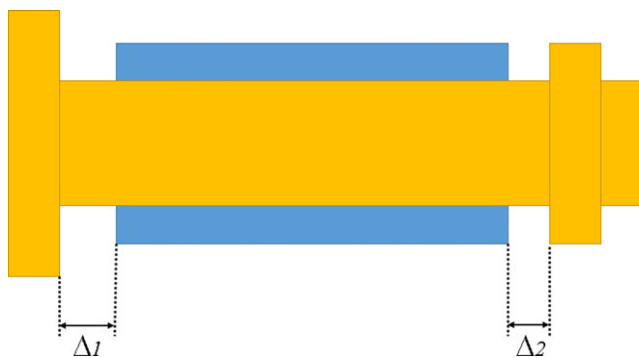
Figure 6. Schematic diagram of the axial clearance.
