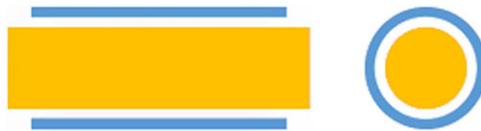
Figure 4. Schematic diagram of the radial clearance.
