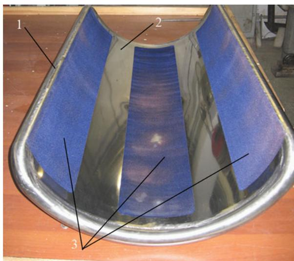
**Fig. 8.** (Color online) Cathode structure: (1) safety frame, (2) cylindrical panel, (3) dielectric emitting surfaces.
