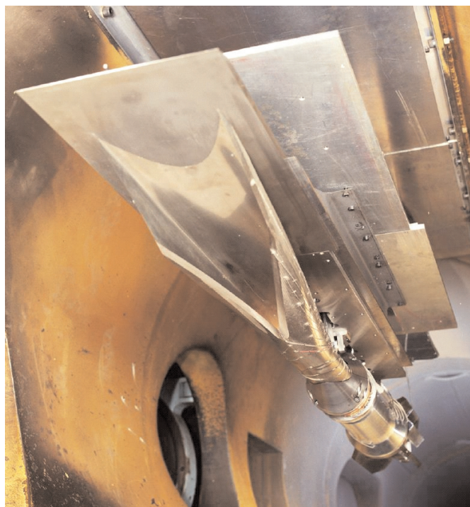
Figure 25. REST inlet model installed in the AHSTF (NASA).
