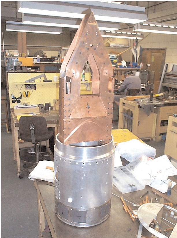
Figure 18. HyShot 2 flight payload.
