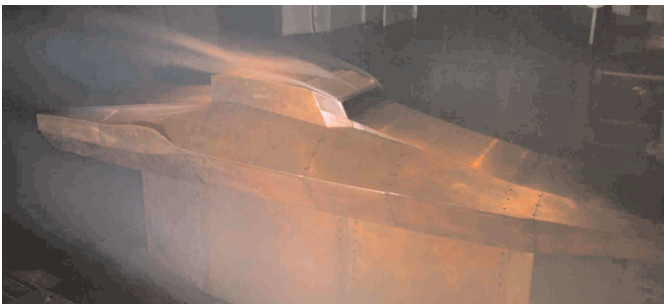
Figure 24. HXFE engine in 8-FT HTT with flow from right to left. (NASA).
