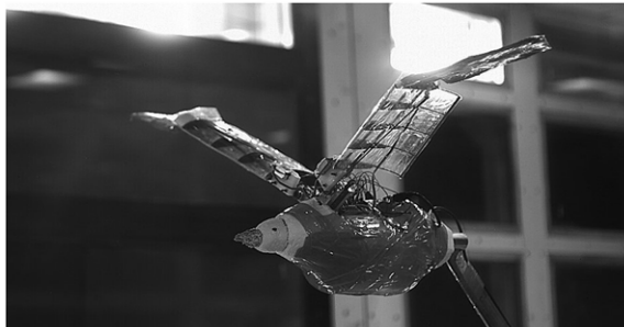
Figure 2. Robogull in flapping action during a wind-tunnel test.
