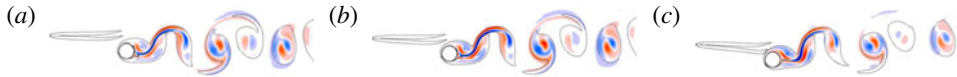
FIGURE 6. Spanwise perturbation vorticity contours at increasing rotation rates, showing the mode C instability with the upstream wire positioned above the cylinder centreline at (-5D, 1D) for Re = 275 . Contour shading is as per figure 4. (a): \alpha = 0.50 , \lambda_z/D = 1.6 ; (b): \alpha = 0.75 , \lambda_z/D = 1.55 ; (c): \alpha = 1.25 , \lambda_z/D = 1.35 .
