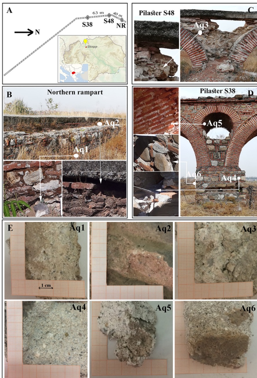
Figure 1 Sampling locations and macrophotographs of samples: (A) a drawing of the overall length (387.98 m) of the Aqueduct and the distance between the sampling locations, along the monument with location of the Aqueduct (drop-like symbol) in Macedonia and location of Macedonia in Europe (inset figure); (B) part of the northern rampart and details of the sampling positions: Aq1 foundation mortar and Aq2 plumbing channel; (C) the ruined Pillar S48 and detail of the sampling position: Aq3-mortar core from the walled opening between the arches; (D) Pillar S38 and details of the sampling positions: Aq4-mortar joint between the bricks (inner layer), Aq5-mortar joint between brick (external layer) and Aq6-mortar joint between the stones/bricks, taken from the surface (external layer); (E) macrophotographs of samples.
