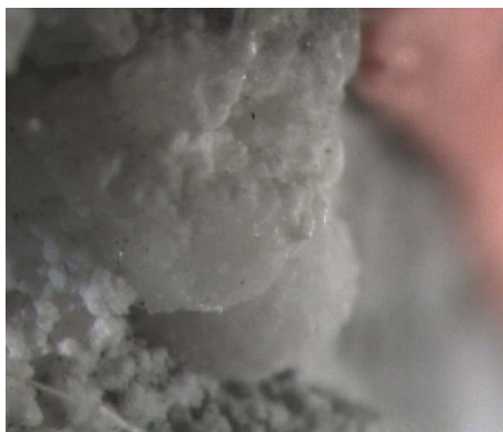
Figure 1. (Color online) Optical image of stromtiodresserite hemispheres embedded in the bulk silicocarbonatite sill rock. The hemispheres are approximately 1 mm in diameter.
