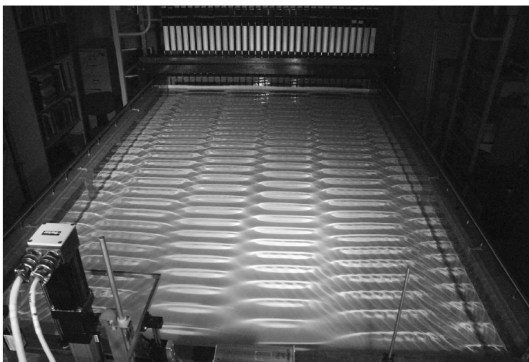
FIGURE 1. Photograph of bi-periodic surface waves with frequency 4 Hz and wavelength in the direction of propagation of about 10 cm.
