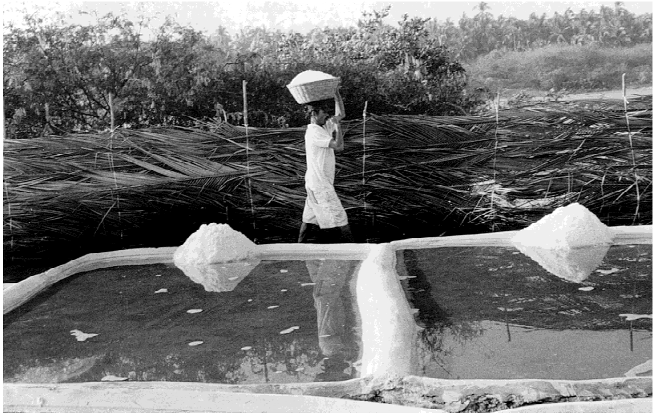
Figure 8. Once the salt has crystallized, it is taken from the era with a basket, or chiquihuite . (Note the mounds of salt in the eras .)
