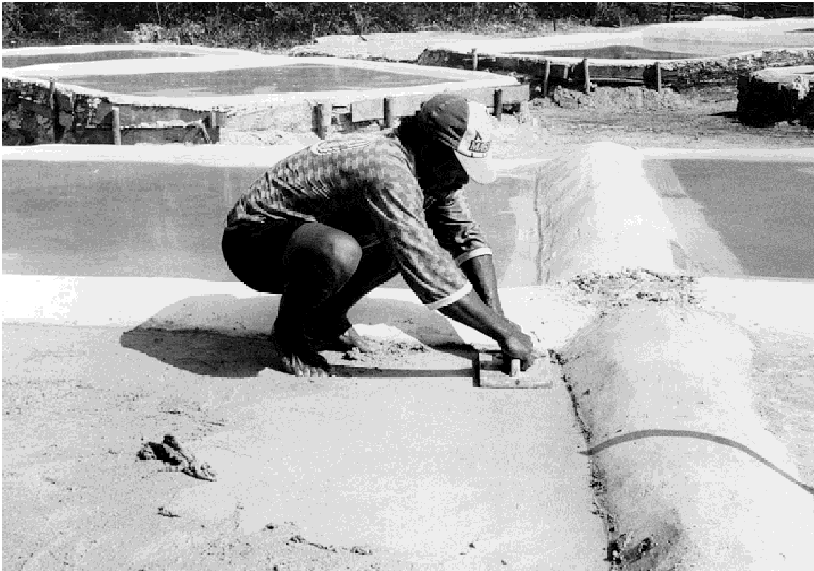
Figure 6. This wooden instrument, known as a menapil , is used to smooth the surface of the era .
