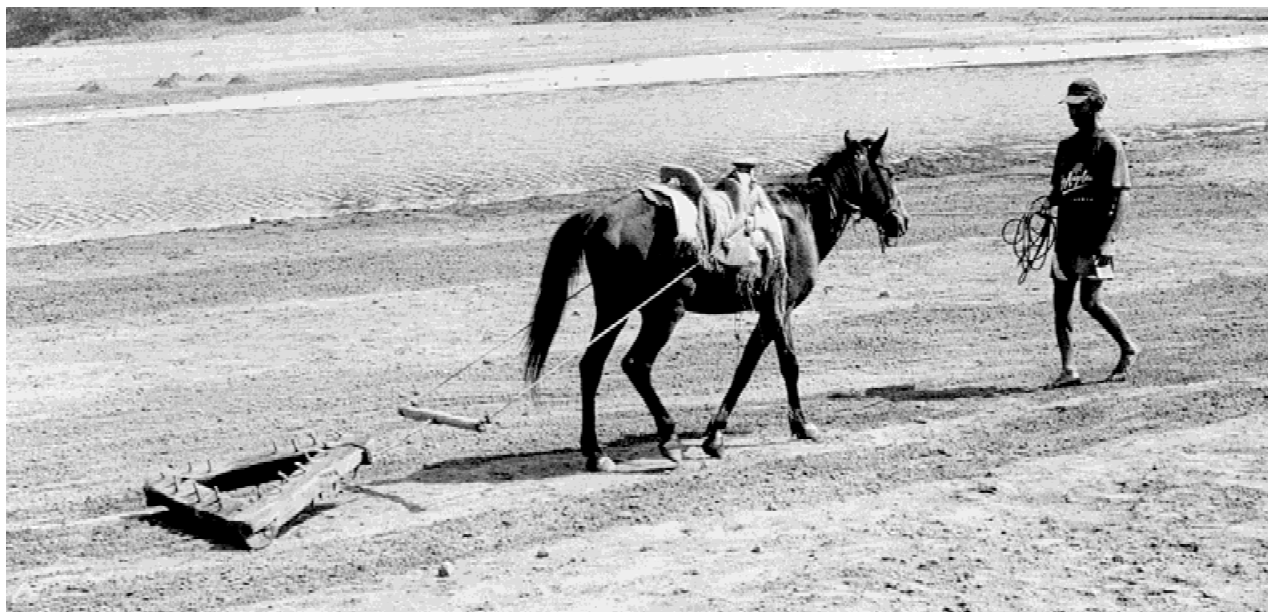
Figure 10. The gata is a wooden implement used to scratch the surface of the soil, making it easier to remove the upper salt-bearing crust.
