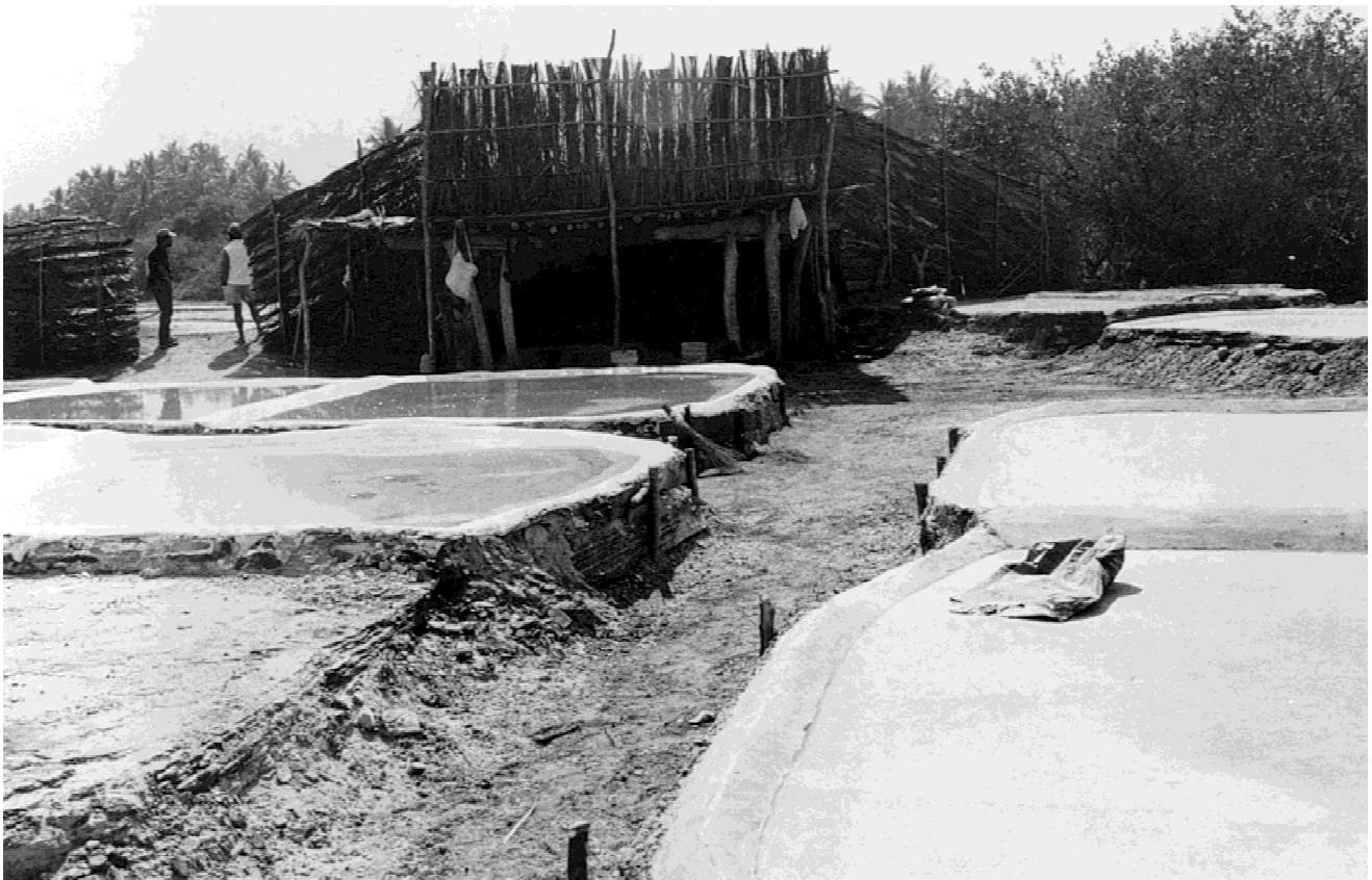
Figure 3. Shallow pools made of sand and lime, known as eras . They are used in the solar evaporation of the brine. The tapeixtle is seen in the back.
