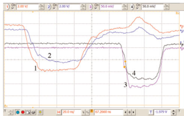
Fig. 15. (Color online) Waveforms of the diode voltage (1), diode current (2), microwave detector signals through the online coupler (3) and in the radiation field (4) (diode voltage 820 kV, diode current 11.4 kA, microwave power 4.4 GW, 20 ns/div).
