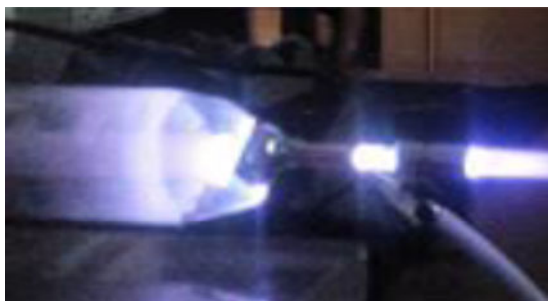
Fig. 3. Cold plasma jet generated using a ring electrode configuration (Divya Deepak et al. , 2016).
