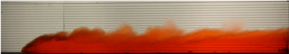
FIGURE 2. Visualization of the gravity current from Exp 6 – see table 1. The current is dyed with food colouring and viewed against a translucent lined sheet.
