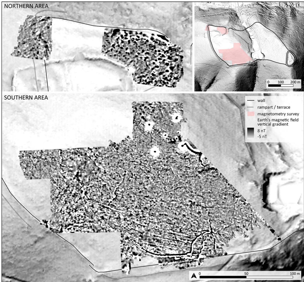
Figure 4. Results of the magnetometry survey. The black dots with white space around them are the results of magnetic anomalies caused by modern metal poles on the top of the hill (figure by authors).
