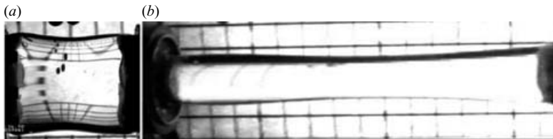
FIGURE 9. Initial and stretched bridge of silicon fluid (liquid 2) at (a) t = 0 and (b) t = 1.344 , respectively; time in dimensionless units.
