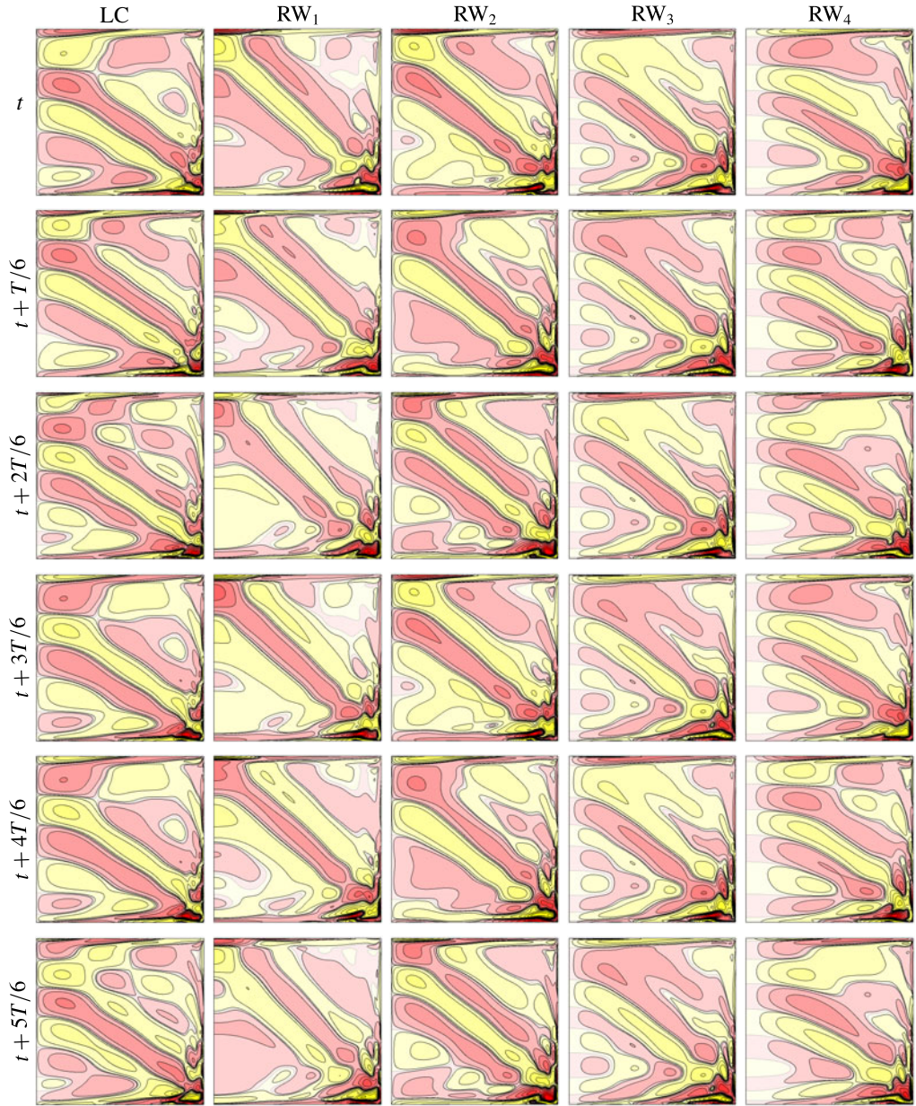
FIGURE 7. (Colour online) Contours of \eta - \langle \eta \rangle \in [-1, 1] for the unstable LC and \eta - \eta_0 for the stable RW_1 , RW_2 , RW_3 and RW_4 in a meridional plane \theta = 0 at Re = 10^4 and Ro = 0.29 ; snapshots at six equally spaced phases over their respective periods are shown.
