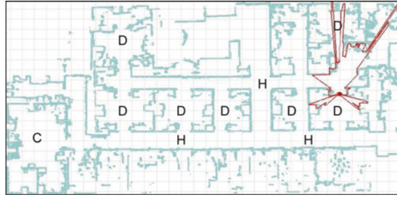
Fig. 3. The map used in experiments. Desk areas, hallways and common areas are marked as “D”, “H” and “C” respectively. LISA’s pose is shown by a red circle and the observed laser reading is shown as a red outline. Note the limited observability LISA in the environment.
