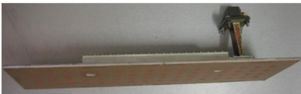
Fig. 14. Prototype of the array ( L = 176 , W = 86 mm).
