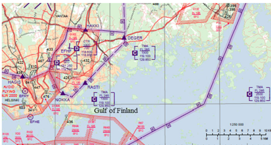
Figure 2. Narrow uncontrolled airspace in the Gulf of Finland (Air Navigation Services Finland, 2017).
