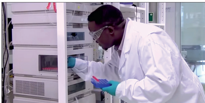
Purification of nanoparticles by high-performance liquid chromatography for pharmaceutical application. Photo credit: Maluta Steven Mufamadi.
