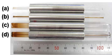
Figure 1. (Color online) Photographs of straight glass monocapillaries: (a) and (b) for inner diameter of 700 \mu\text{m} without and with Au coating, respectively; (c) and (d) for inner diameter of 400 \mu\text{m} without and with Au coating, respectively.
