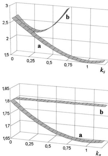
Fig. 6. Absolute increment in joint torques depending on the step size.
