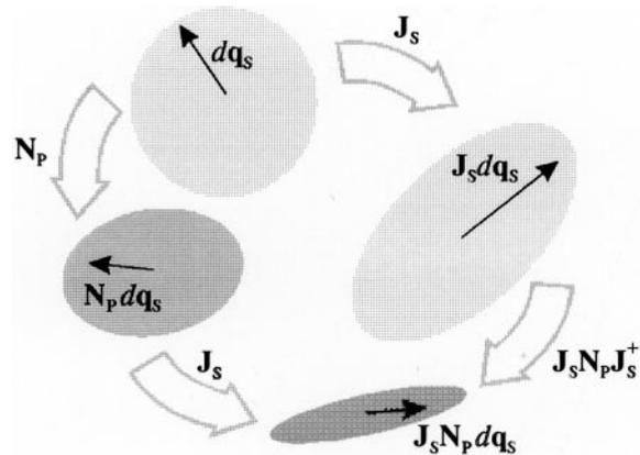
Fig. 1. Manipulability ellipsoid mapped in the null space of the primary task.
