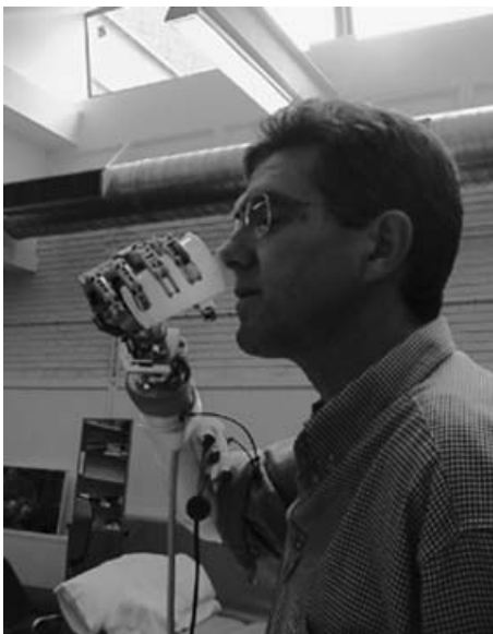
Fig. 1. One of the MANUS users performing a combined cylindrical grasp and wrist rotation.
