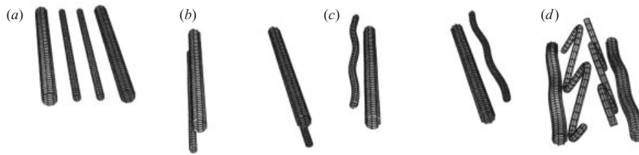
FIGURE 3. Optimal perturbation computed for X/b_0 = 30 in the case \Gamma_2/\Gamma_1 = -0.3 , b_2/b_1 = 0.3 . (a) X/b_0 = 0 , (b) 10, (c) 20 and (d) 30.
