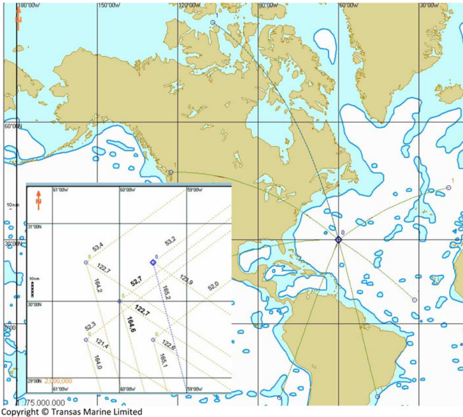
Figure 10. Using ECDIS (Transas, 2010) to plot GP and Azimuths-Example 1.
