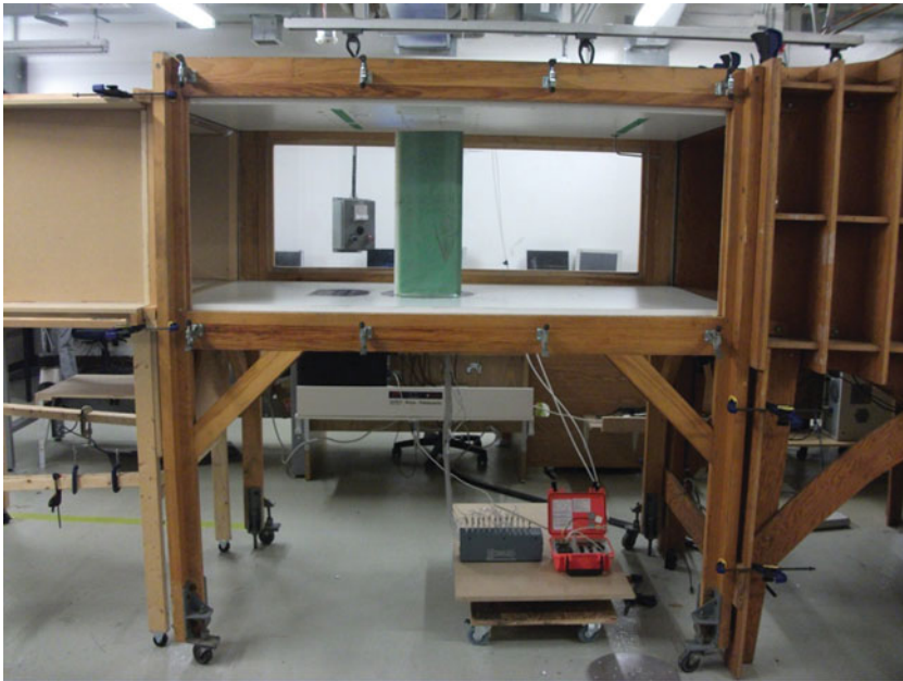
Figure 5(b). (Colour online) Original rigid wind model installed in the wind-tunnel test chamber and connected to the AEROLAB measurement system.
