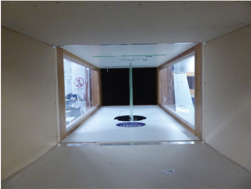
Figure 5(a). (Colour online) Optimised wing model installed inside the test chamber ready for testing.
