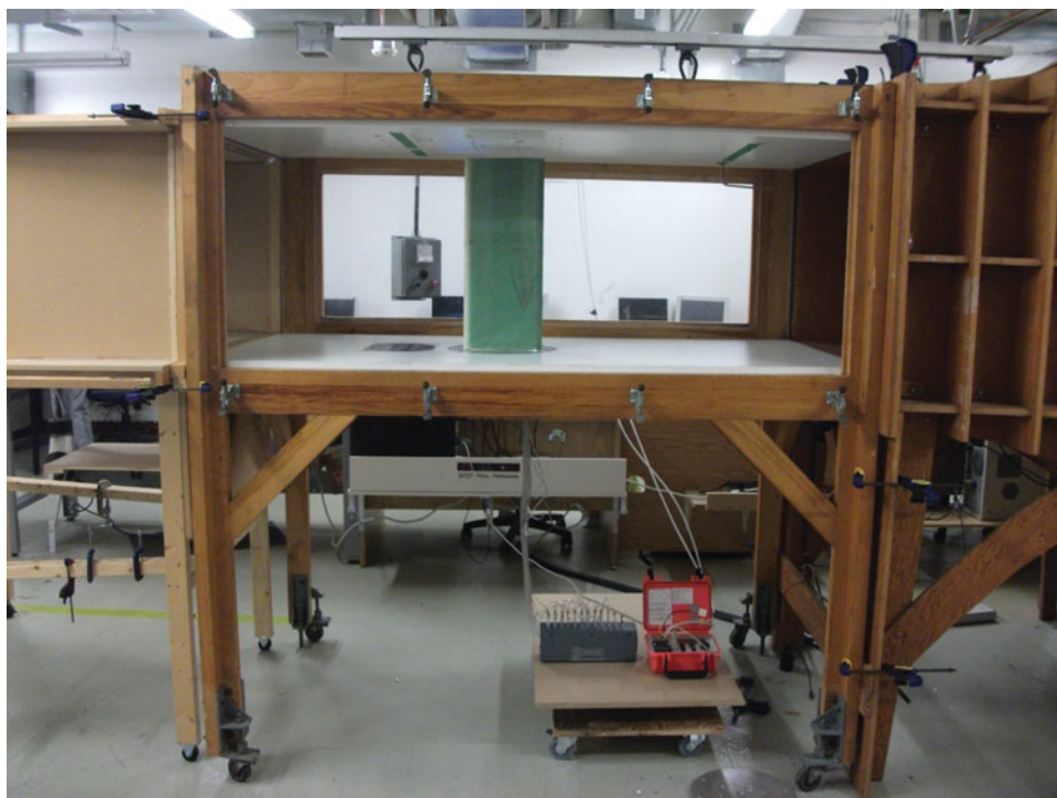
Figure 4a. (Colour online) Wing model installed in the wind-tunnel chamber.
