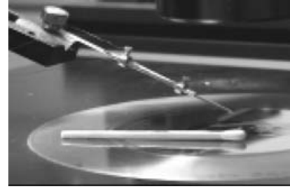
Fig. 3. Photograph of touch sensor with the pipette.
