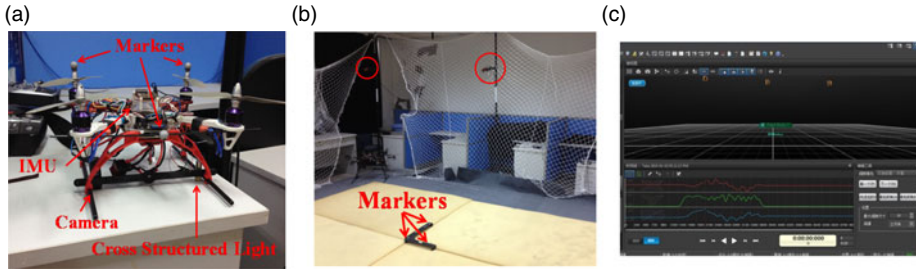
Figure 8. The environment of verification. (a) The quad rotor test bed designed independently. (b) The easy track motion capture system. (c) The screenshot of motion capture system software.
