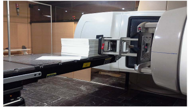
Figure 3. Set up of film to achieve profile and percentage depth dose (energy 6 MeV, Varian Linac accelerator, SSD = 100 cm, FSD = 10 × 10 cm).
