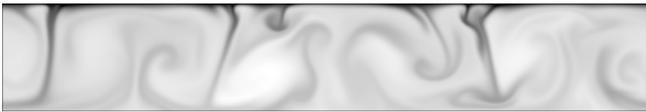
FIGURE 3. Instantaneous temperature field from a two-dimensional simulation of our model with R = 1.44 \times 10^8 , Pr = 1 , a horizontal period of 6 and no-slip boundaries. The hottest fluid (white) is 0.06 dimensionless degrees warmer than the coldest fluid (black).
