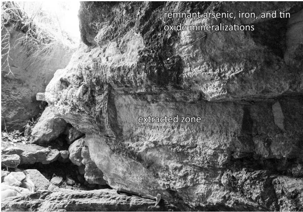
Figure 2. Gallery wall at Senir Sırtı Kerim household showing extracted zone and remnant arsenic, iron and tin oxide mineralisations; photograph by J.W. Lehner.
