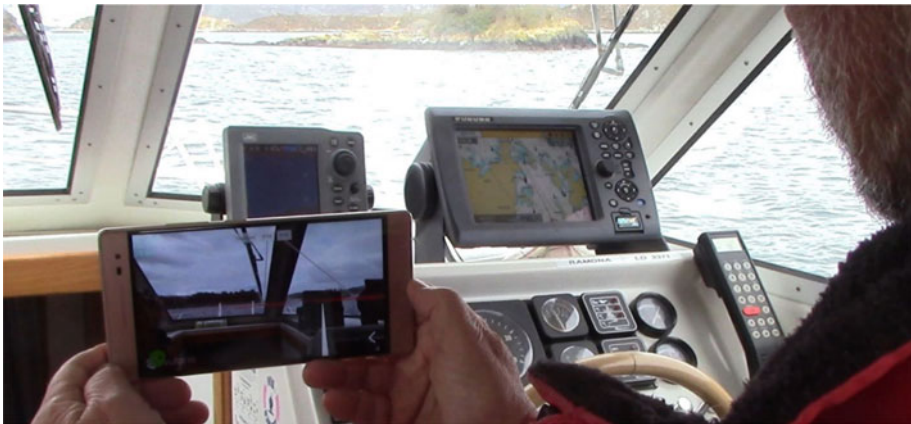
Figure 4. The test application on the smartphone (Lenovo Phab 2 Pro) during the pilot test. To the right is the boat’s reference fixed chart plotter.
