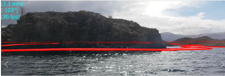
Figure 8. The picture shows the offset of the AR layer with the red NoGo areas. There is a vertical offset and a horizontal and fluctuating offset due to noise in the phone's internal compass. However, users judged it acceptable during the tests.
