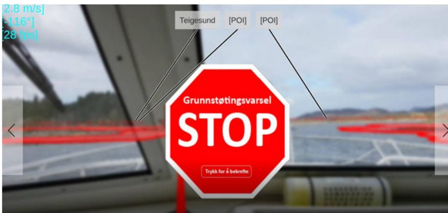
Figure 6. Screen dump from the Galaxy test phone. The grounding alarm has been triggered with both an aural and a visual alarm.
