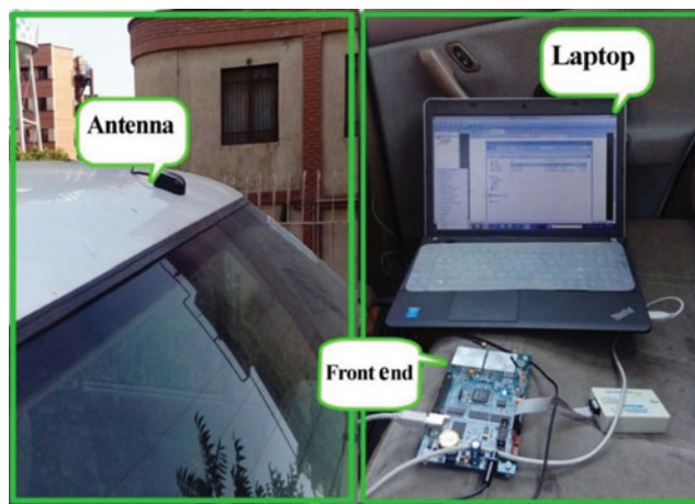
Figure 10. Setup for recording real data around Iran University of Science and Technology.
