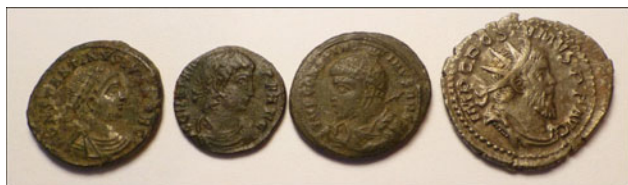
Figure 8. (Color online) Silver-washed (far left) and silver coated (far right) coins. The middle two coins have nearly identical phases and silver content to the silver-washed coin. These coins correspond to #17, #15, #12 and #4 in Table I.
