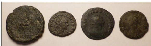
Figure 4. (Color online) Four Roman coins exhibiting bronze disease. All four have high concentrations of CuCl. These coins correspond to #1, #6, #8 and #9 in Table I.
